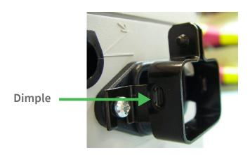
Clamp: The clamp has two dimples inside it on both sides. The purpose of the dimples is to squeeze on to the shoulders of the power cord and secure it within the socket (after the power cord is inserted fully into the socket and seated correctly.
